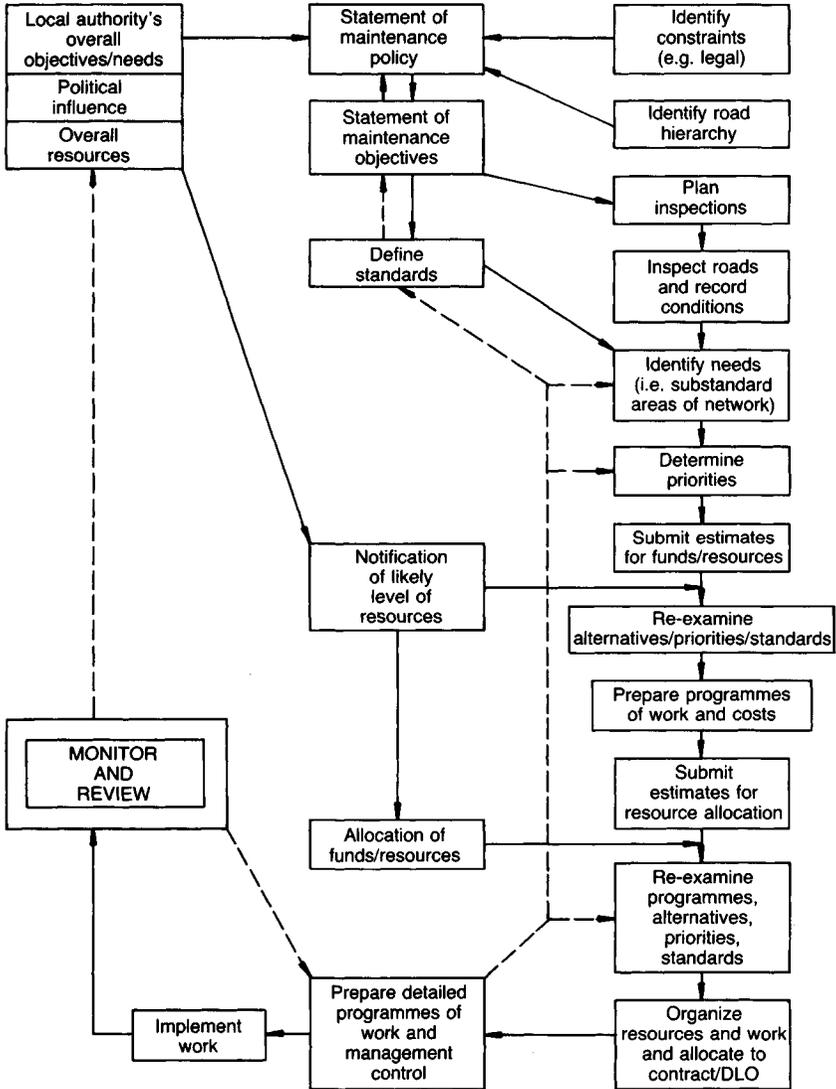
Fig. 1.3. Maintenance management flow diagram
